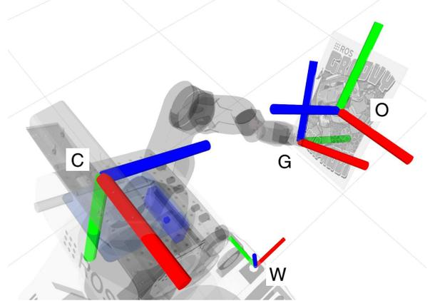
Fig. 2. Coordinate frames referred to in the (A) actuated and (B) static camera scenarios:  $A$  = arm,  $C$  = camera,  $O$  = calibration object,  $W$  = world or robot, and  $G$  = gripper tool frame. In scenario (A) the goal of the calibration procedure is to estimate the transform between camera and arm,  $\mathbf{T}_{AC}$ , and in scenario (B) the goal is to estimate the transform between camera and world,  $\mathbf{T}_{WC}$ .
