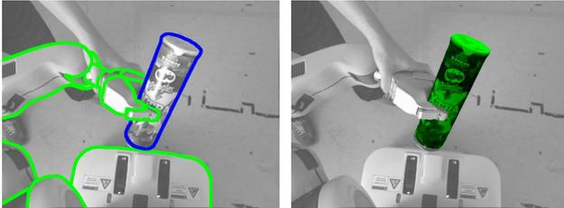
Fig. 3. (A) Blue outline shows the object pose as estimated through vision-based pose estimation and green outline shows the robot pose as obtained from the joint angle measurements. (B) Object appearance as predicted from the estimated object pose and a textured wireframe model of the object. The texture is overlaid in green and does not contain the specular reflections in (A). The region occluded by the robot is also correctly discarded.
