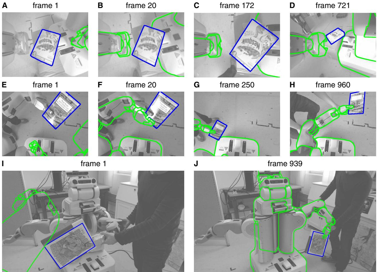
Fig. 5. Snapshots from the on-line calibration procedure applied to real-world sequences involving an actuated camera (A–D), a static camera on the robot (E–H), and a static camera external to the robot (I–J). The robot’s right arm is not shown in panel (J) since it was broken at the time of the experiment and the joint encoder offsets were unknown. The full sequences are shown in the *Supplemental Material Video*.
