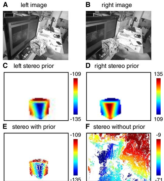
Fig. 3. (A) Left and (B) right input images and low-resolution (C) left and (D) right stereo priors generated using the previous frame pose estimate of the manipulated box. (E) Stereo obtained using four scales and initializing with the prior, and (F) stereo obtained using six scales and without using the prior.
