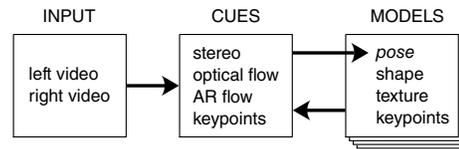
Fig. 1. Method overview illustrating the different visual cues (AR = augmented reality, see II-B2) and model components. The cues are combined to estimate the objects poses and scene information is fed back to facilitate the cue extraction.
