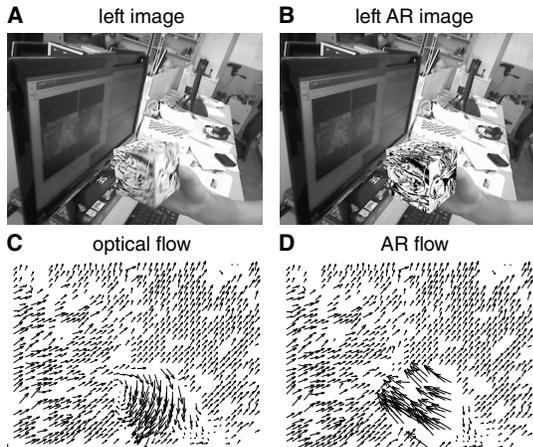
Fig. 4. (A) Left image and (B) left image with rendered model (at incorrect pose) superimposed. (C) Real optical flow from real image in A to the next real image. (D) AR flow from AR image in B to the next real image. Both flow fields are subsampled ( $15\times$ ) and scaled ( $5\times$ ).
