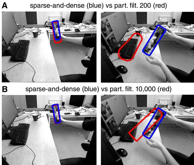
Fig. 15. Comparison between *sparse-and-dense* and the *particle filter* method on a real-world image sequence. In the left column (A to B) we see the improved accuracy that results from increasing the number of particles. In the right column we see the failure of the *particle filter* method due to high speed object motion and motion blurring. These images are representative snapshots of much longer sequences (see *Supplemental Material Video 4*).
