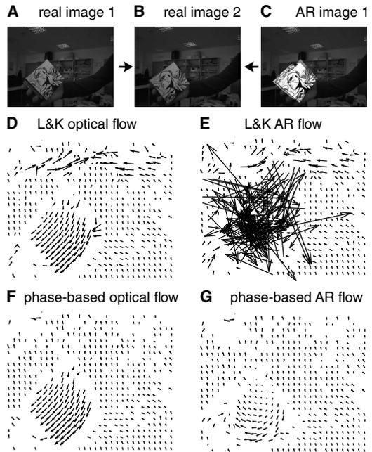
Fig. 5. Importance of intensity invariance for AR flow computation. (A) and (B) are consecutive images obtained with short exposure. The AR image (C) is composed by superimposing the model (with much brighter texture) at an incorrect pose on image (A). Optical flow from A to B computed with (D) pyramidal Lucas & Kanade and (F) our phase-based algorithm. AR flow from C to B with (E) pyramidal Lucas & Kanade and (G) phase-based. All flow fields are subsampled ( $20\times$ ) but unscaled.
