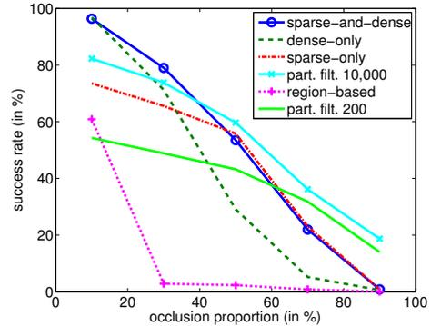
Fig. 12. Average tracking success rates obtained across all benchmarking sequences as a function of the proportion of the tracked object that is occluded.
