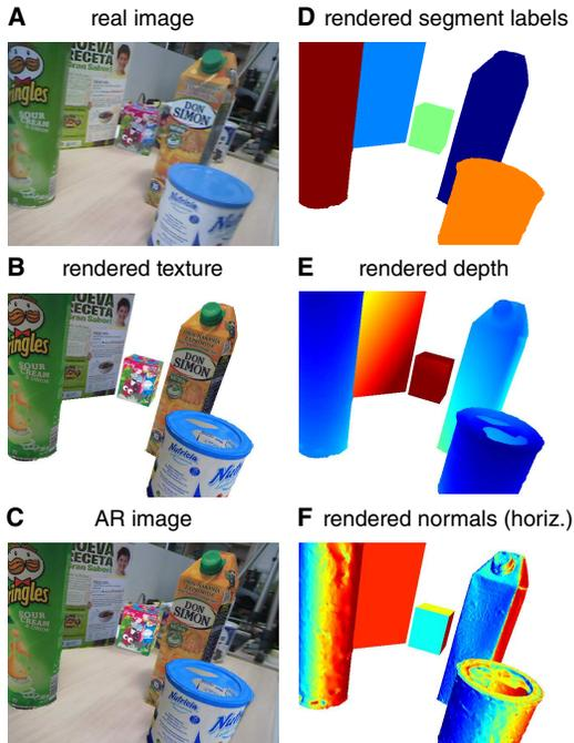
Fig. 2. (A) Original input image, (B) color image obtained by rendering the textured models according to the current pose estimates, (C) AR image obtained by merging A and B (see II-B2), (D) segment (object identity) labels accounting for occlusions, (E) depth-buffer, and (F) horizontal component of the normals. Note the model errors in the lid of the *Nutricia* object.
