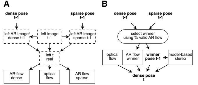
Fig. 6. Combined sparse pose detection and dense pose tracking. Dashed boxes refer to images and solid boxes to extracted cues. (A) Processing sequence for obtaining the three different motion cues. (B) Sequence performed to obtain the dense cues and select the winner pose. Note that model-based stereo only needs to be computed once since it is not used in the evaluation.
