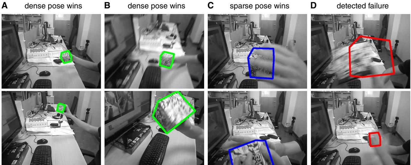
Fig. 13. Indicative real-world single object pose estimation results, showing how the dense pose is selected when (A) the object is far and/or (B) motion-blurred, how the sparse pose is selected in case of (C) strong occlusions, and how (D) failures can be detected correctly.
